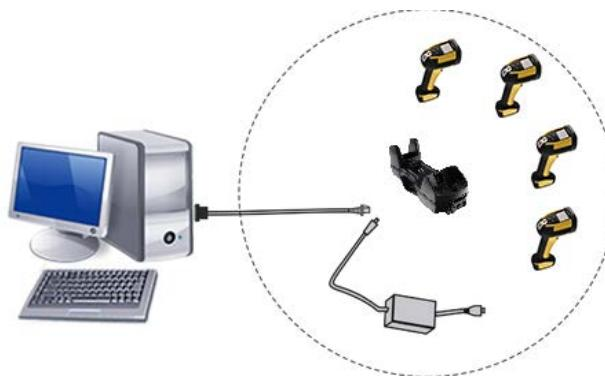
In stand alone systems, each base station is connected to a single Host.
