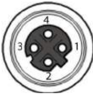
Figure 3 – M12 D-Coded Female Ethernet Network Connector
