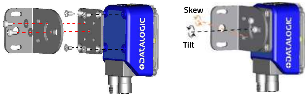
Figure 5 - Positioning with Mounting Bracket
