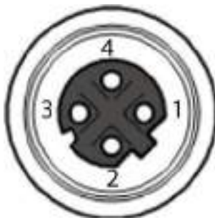
Figure 2 – M12 D-Coded Female Ethernet Network Connector
