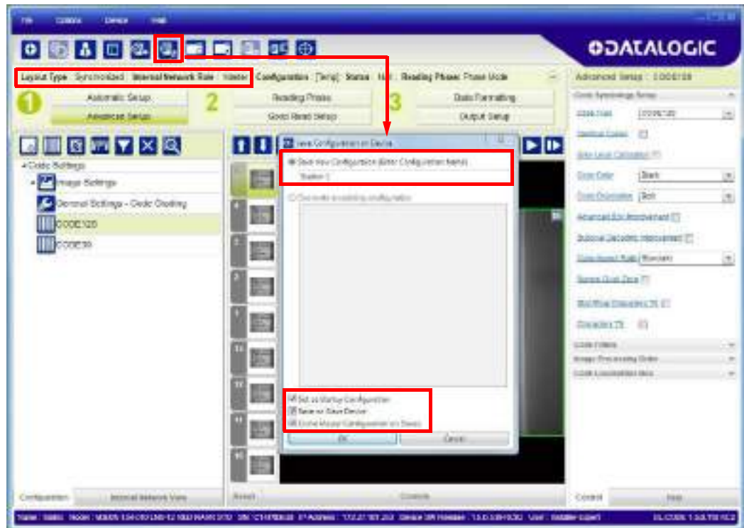
Figure 96 - Saving Synchronized Phase Mode Configuration to Master
