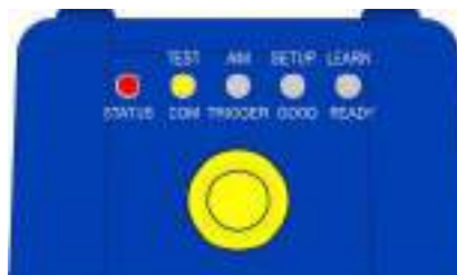
Figure 13 - X-PRESS Interface: Test Function
